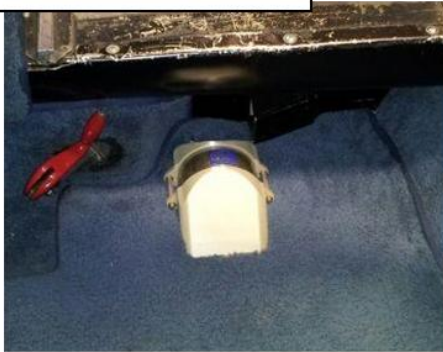
Location of installation for a blower in a V35
